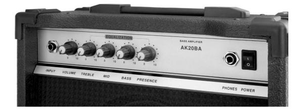
Volume: This knob can be used to adjust the volume in the clean channel
