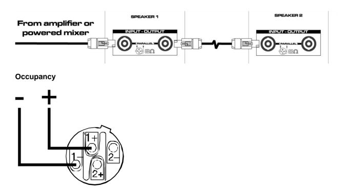
**1. Input:** This input allows you to connect an active speaker to your passive speaker using Speakon compatible speaker cable.
