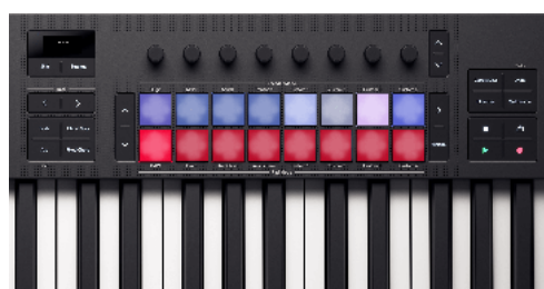
The Launchkey 49 pads reflecting the track select and record arm states on the pads.
