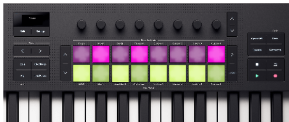
The Launchkey 49 pads reflecting the mixer Mute and Solo states on the pads.
